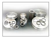
Pistons and glands are made of aerospace grade 6061 T6 aluminum to reduce weight and the possibility of corrosion. Tie rods, where applicable, are made of 304 stainless steel. The main rod (shaft) is generally nitrided or hard chrome plated; but other materials are available.
