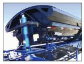
With bore sizes available from 1.5" to 16", over 100" of stoke depending on diameter, and up to 5000 PSI operating pressure, we've got your hydraulic cylinder needs covered.
