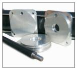
All processed parts, with the exception of some rod end mounts, are precision CNC machined. Piston and aluminum ends are made of aerospace grade 6061 T6 aluminum. Tie rod material is 304 stainless steel. Nitrided steel, which has excellent dent and corrosion resistance, is used for the main rod (shaft). Hard chrome plated is also available.
