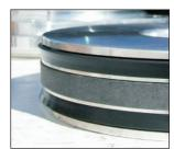
U-cup seals, which are standard on our composite tube cylinders, provide less friction than traditional o-ring seals. Lip design removes contamination versus o-ring seals that tend to rub particles into the cylinder wall. U-cup seals offer improved sealing properties and increased
